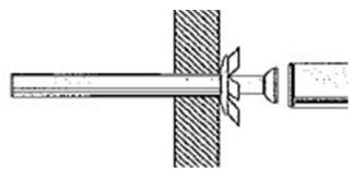
For use with walls stuck with plaster board. The hammer fixing allows it to be fixed to the wall rather than the plaster board. Always check the fixing is secure to the retaining wall.
