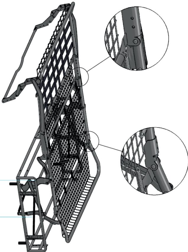
It is also important to lubricate the joints correctly.
