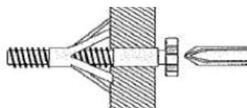
For use with plaster board partitions or hollow wooden doors.
