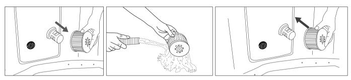
**NOTE:** Change the filter cartridge every 3-5 days, or if the filter cartridge remains soiled and discolored. **NOTE:** When the spa is filled with water, there should always be a filter cartridge installed on the base. **NOTE:** Turn off all the functions before changing or cleaning the filter cartridge.
