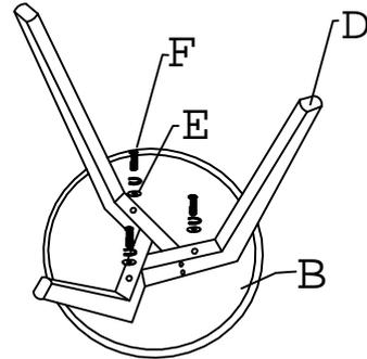
Do not tighten the screws completely until all screws are connected.
